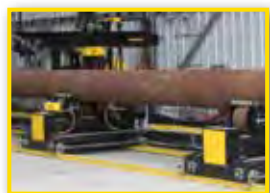
Rail-mount base - can be supplied as motorized or non-motorized for driving pipe sections together
