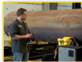
Alignment, leveling and high/lows easily adjustable using pendant or touch screen control
