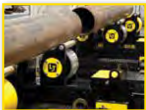
Pipe loaded, lined up using track drive
