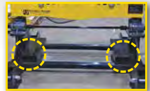
Forklift pockets for safe & easy transportation
