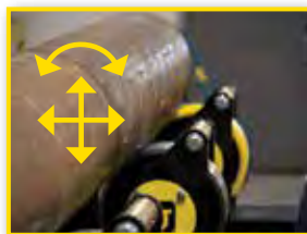
Alignment, side shift, and leveling functionality
