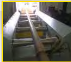
Large bore conveyor for up to 40" OD pipe
