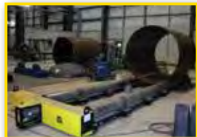
Modular construction allows for multiple lengths to be added for longer vessels
